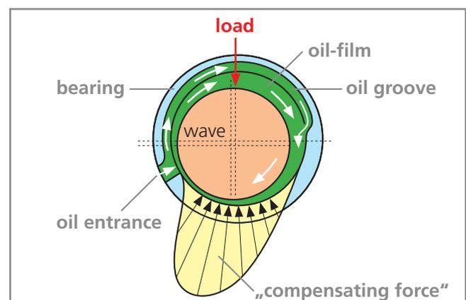
Picture 2: The load-spread in a plain bearing
